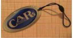
Hitag μ Anhängerschlüssel / Keyfob                        | 125 kHz / 134.2 kHz  | NXP  | R / W, 1760 bit   | Up to 8            | ISO 11784/85    |
