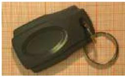
Hitag μ Anhängerschlüssel / Keyfob                        | 125 kHz / 134.2 kHz  | NXP  | R / W, 1760 bit   | Up to 8            | ISO 11784/85    |
