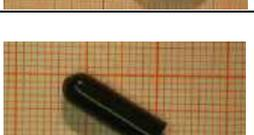
Hitag μ Glas-Transponder 5 x 16 mm / Glass transponder  | 125 kHz / 134.2 kHz  | NXP  | R / W, 1760 bit   | Up to 8            | ISO 11784/85    |
