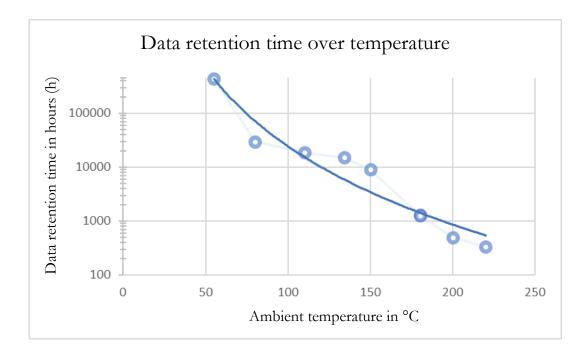
There is usually no clear information from the RFID IC manufacturers on the data retention time when the specified temperature of  $+55^{\circ}$  C is exceeded. The information we provide on the data retention time is based on internal investigations in which our transponders are used at increased ambient temperatures and on technical statements by the chip manufacturers. The values stated are guide values and serve as orientation.
