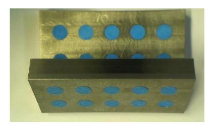
After the test, all tested transponders could be read out without any problems!
