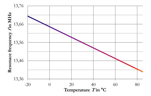
The typical resonance frequency of 13.56 MHz occurs at room temperature. The resonance frequency increases with lower temperatures. With higher temperatures, the resonance frequency drops.
