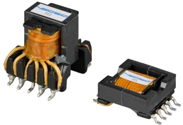
Figure 3 – Customised transformers made from standard components
